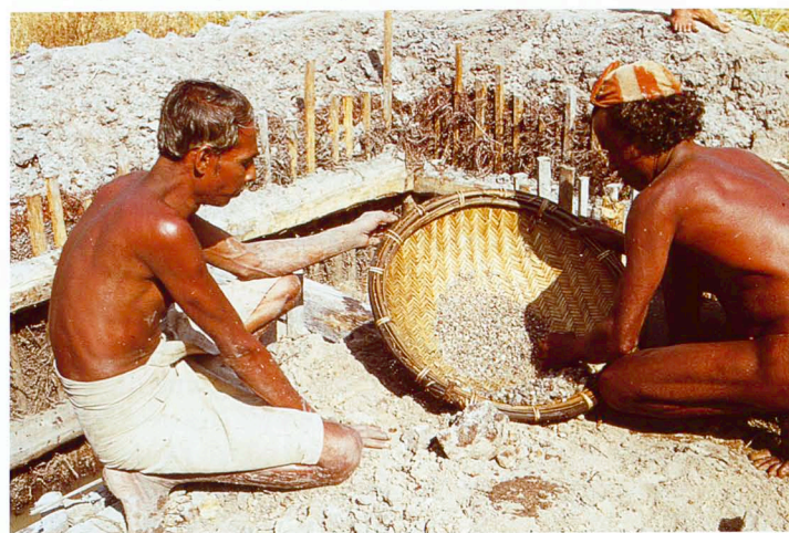
Figure 16. After washing of the illam (gem-bearing gravels), miners in Sri Lanka examine them for gem rough. Today, these time-honored recovery methods are still used by many gem miners in Sri Lanka and elsewhere. Photo by Edward J. Gübelin, from the early 1960s.
