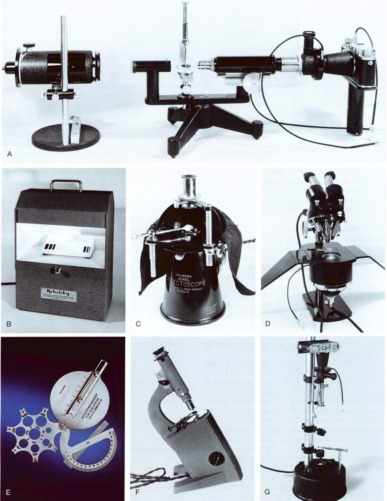
Figure 17. Dr. Gübelin developed a number of diagnostic gem-testing instruments during the 1940s and '50s, including: (A) the horizontal immersion photomicroscope, (B) the Koloriskop, (C) the Detectoscope, (D) the Gemmoscope, (E) the cut measuring device, (F) the Jewelers' Spectroscope, and (G) an innovative device that allowed the user to magnify and then photograph a gem's spectrum. With the exception of photo E, which was taken by Harold & Erica Van Pelt, all the other photos were commissioned or taken by Dr. Gübelin shortly after the development of the instrument.
